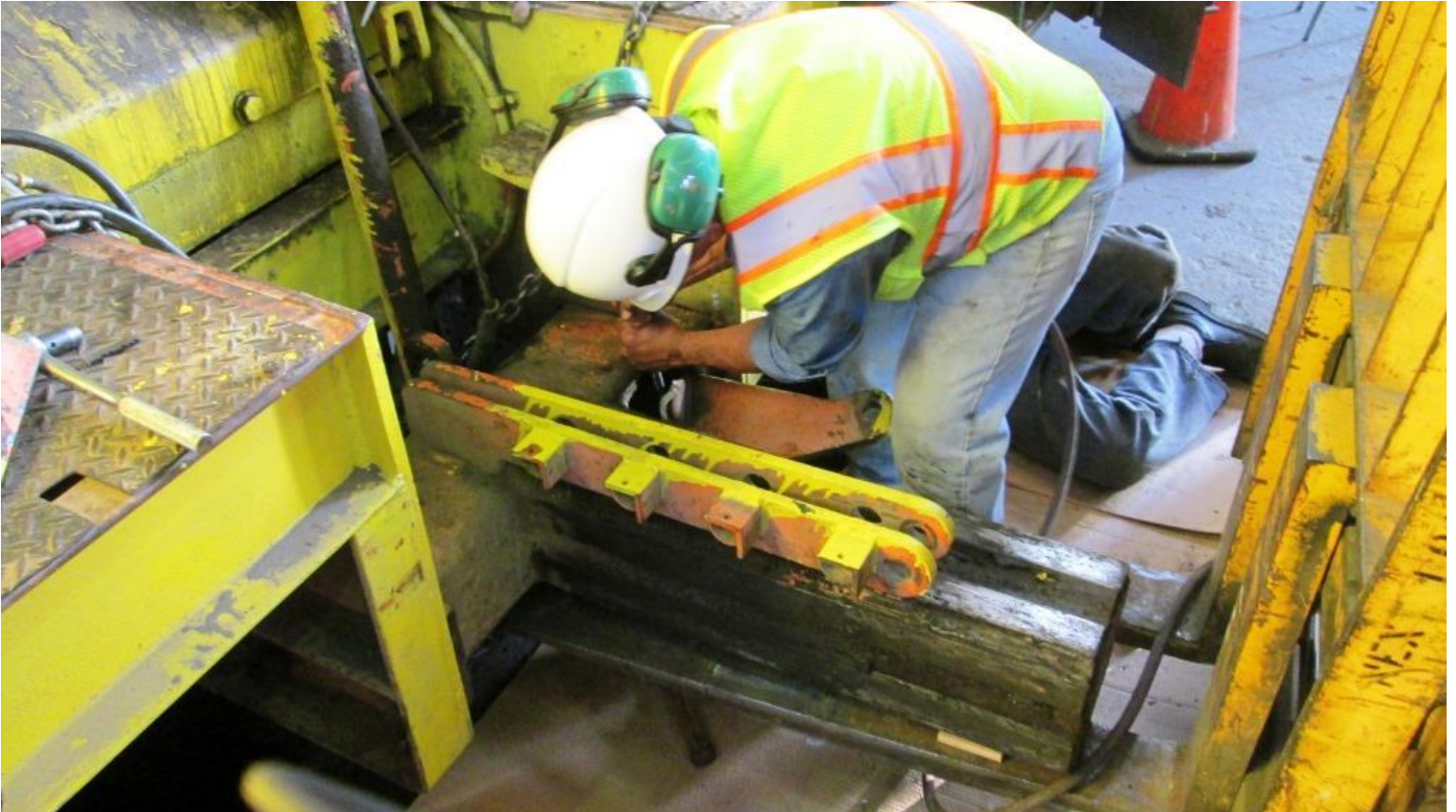
Joe holds the nut on tight with a ratchet as Fred (legs) uses the impact-wrench under the machine to remove the bolt
