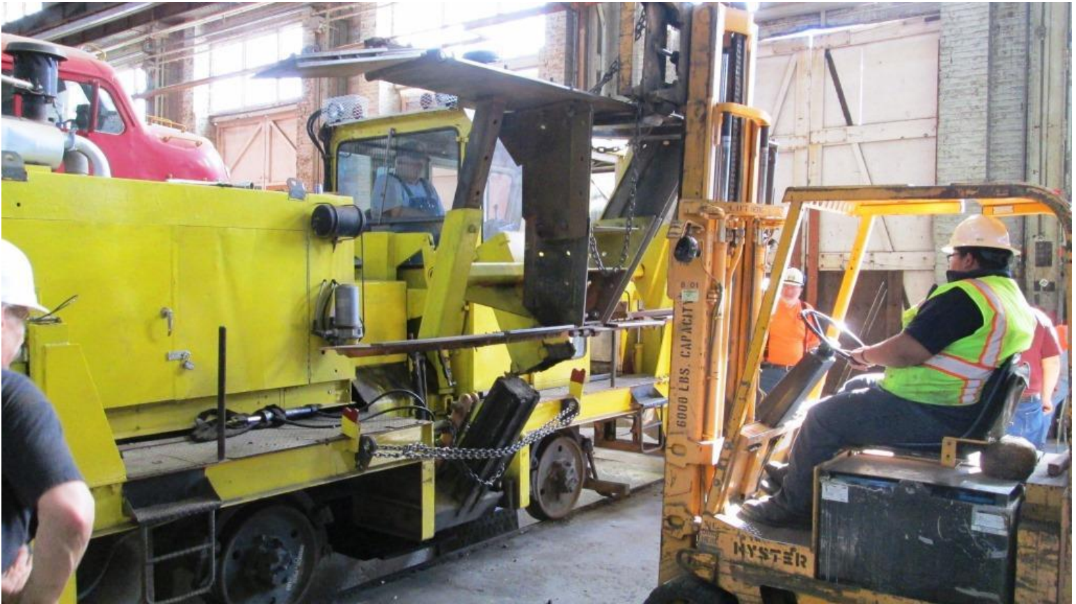
Anthony on the forklift gingerly removes the wing from the regulator as Frank, Gene, Pat, and Fred provide guidance
